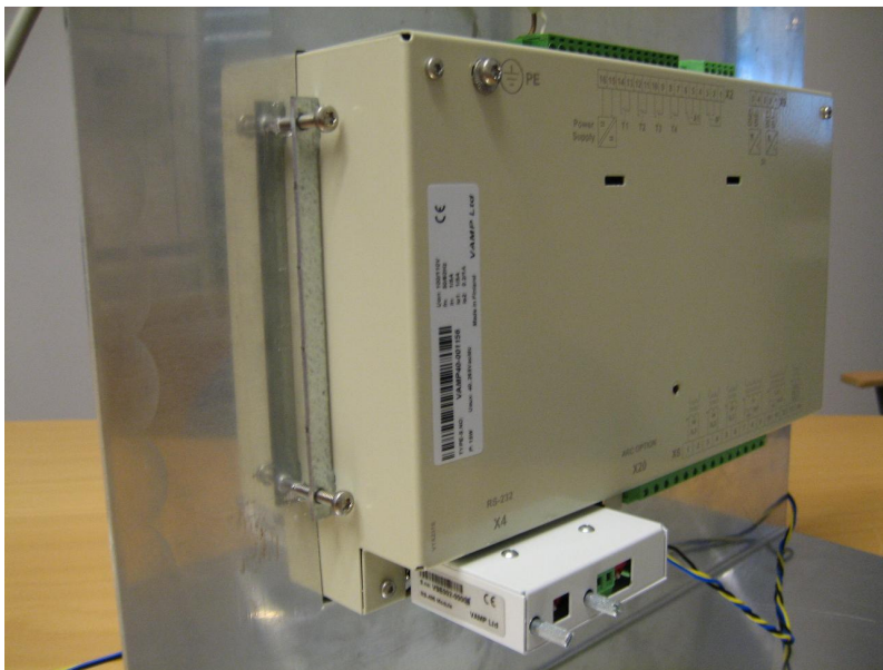
Figure 5. VSE 002 is attached to VAMP 40
