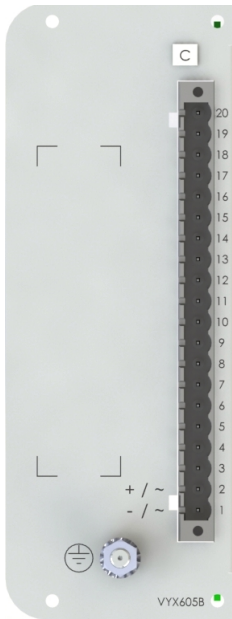
Figure 10.2: Example of supply voltage card Power C 110-240
