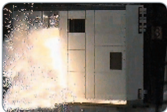
Traditional protection relay systems do not provide fast enough protection in arc-fault situations.
