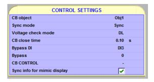
5) Set your settings for the synchrocheck i.e. the maximum allowed frequency, phase angle and amplitude differences.
