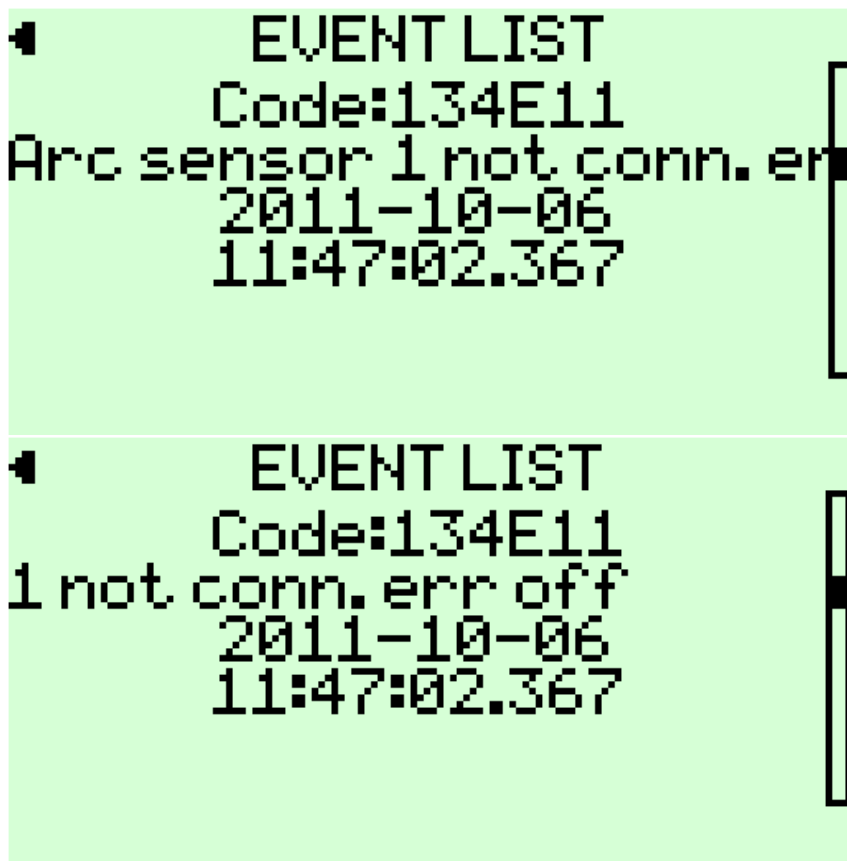
Figure 18: 'Arc sensor 1 not conn. err off'
