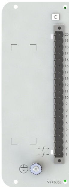
Figure 10.2: Example of supply voltage card Power C 110-240
