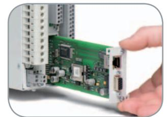
The optional DI/DO, arc connection and communication modules can be added to the basic relay later on in order to extend the functionality of the relay during its life time without firmware update.
