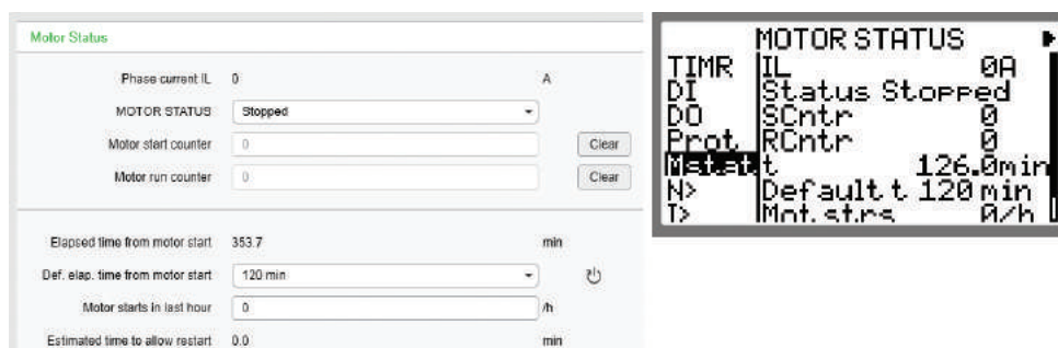
Figure 93 - Motor status via Easergy Pro and local panel
