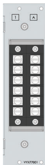
Figure 208 - Analog measurement card "1 = 3xI (5/1A) ring lug + Io (5/1A)"
